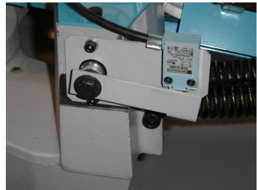
Cutoff actuator shown, adjusted for cutoff position with sawframe down
